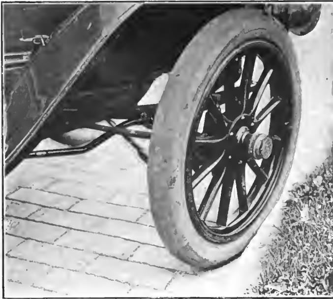
Fig. 1—Outer wheel of the automobile strikes the curb in the process of turning the car around, injuring the fabric beyond repair
